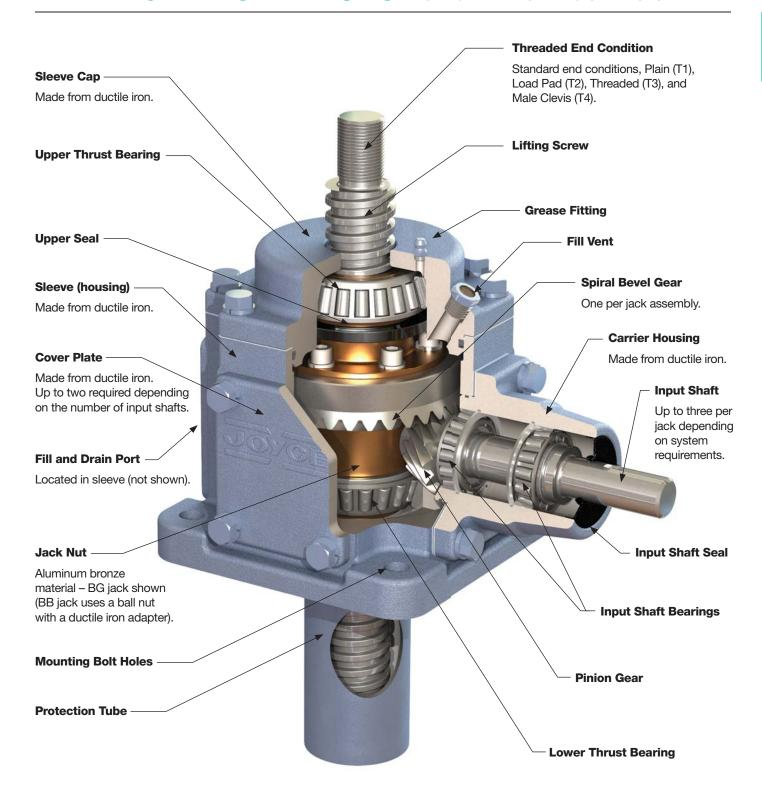
This graphic shows a Joyce Bevel Gear® jack (BG). Bevel ball actuators (BB) also use a bevel gear set. See pages 148 - 167 for more information.
