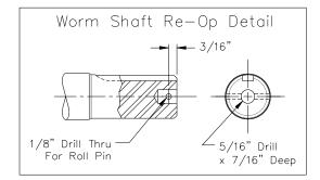
When field mounting limit switches it is important to be sure the jack worm shaft is machined to allow proper mounting of the limit switch housing.
