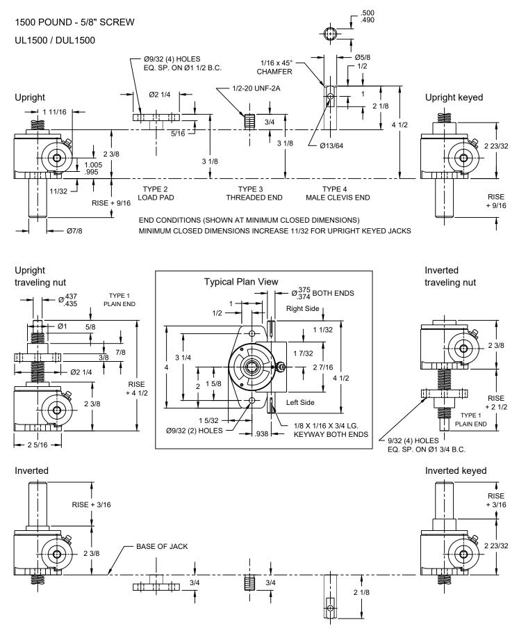
Material Notes: Housing and protection tube are aluminum. Lifting screw is cold drawn steel (CDS). Input shaft (worm) is CDS. Note: Drawings are artist's conception - not for certification; dimensions are subject to change without notice.
