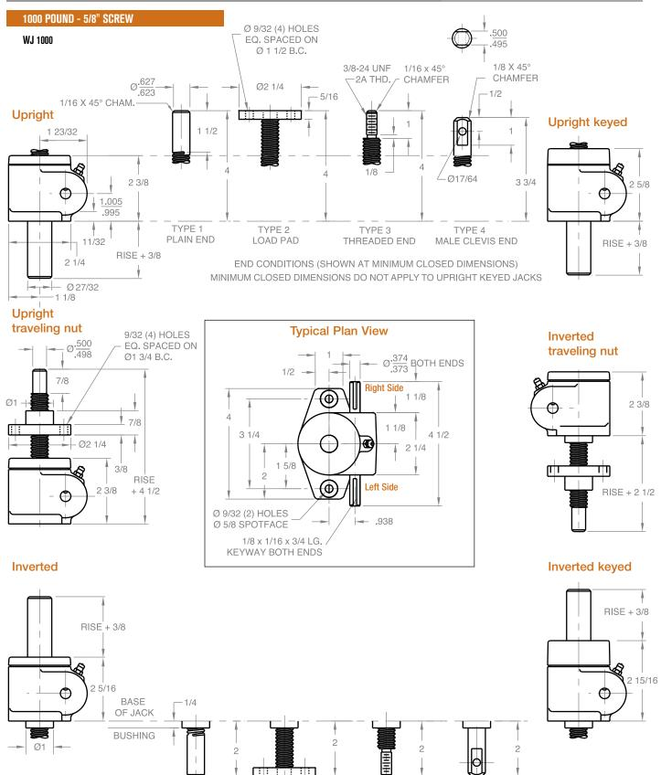
Material Notes: Housing and protection tube are aluminum. Lifting screw is 304 S.S. Input shaft (worm) is 416 S.S. Note: Drawings are artist's conception — not for certification; dimensions are subject to change without notice.
